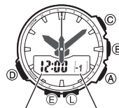
Alarm time (Hour : Minutes) Alarm number
